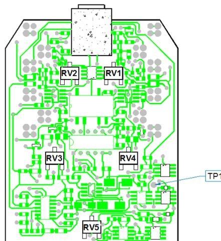
To calibrate the temperature output for a module configured for a 10mV/ $^{\circ}$ C sensor, the milli-ammeter is connected to terminals M and J. With no input signal applied the output current can be set to 4.0mA using potentiometer RV2. A dc voltage corresponding to the maximum temperature (eg. 1.0V = 100 $^{\circ}$ C) is then applied to terminals C and F. The output current can then be adjusted to the maximum 20.0mA using potentiometer RV4.
