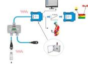
We offer a full line of equipment for permanent machine protection systems. The HS-530 and HS-535 are modules that provide accelerometer power and condition the signal to provide 4-20mA output, proportional to acceleration or velocity. Also available is a buffered AC signal via the front panel which can be used by a data collector. The HS-510 vibration trip module can be used to provide an alarm based on user preset warning and alarm levels.
